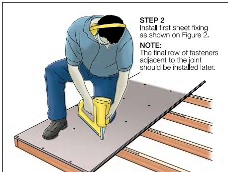
FIGURE 5 FIXING 1ST PANEL
